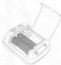
Two batteries in the left two banks.
