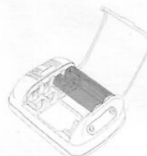
Two batteries in the right two banks.
